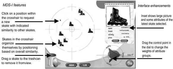
Figure 2. MDS-Interactive interface to a database of roller skates (design: Bram van den Nouweland).
