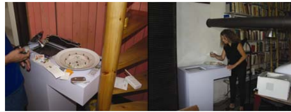
Figure 2: working prototypes in home situation (left: son's home; right: mother's home). Each prototype contains a camera, motor and sensor, a bowl, display, and internet-linked personal computers.
