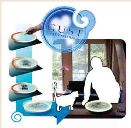
Figure 1: Operation of the gustbowl: throwing in the keys causes a bowl to wobble. A picture is taken and sent to the other bowl, which wobbles in turn, and displays the picture.
