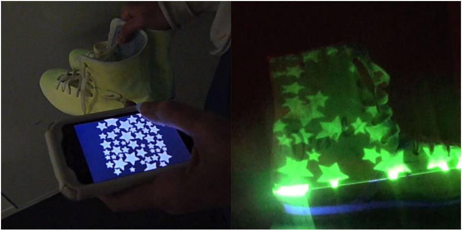
Figure 8.3. The Slow Display is a projector display that has high resolution but a very slow frame-rate. Once objects or surfaces are written, the color change sticks for minutes, hours and potentially days.
