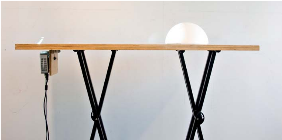
Figure 5.8. The light from the projector is reflected by a mirror and goes over the table, illuminating only the objects on the table. The light that is not blocked by objects, is washed out by a light source stronger than the projector. A few prototypes of the Object table are depicted. On the bottom, the table with integrated projector. The light is projected through a hole in a small mirror (top left). Alternatively the projector can be attached to any table to make use of available tables on location. Top right shows the projector mounted to the side of a table, with the mirror is then attached to the projector using velcro.
