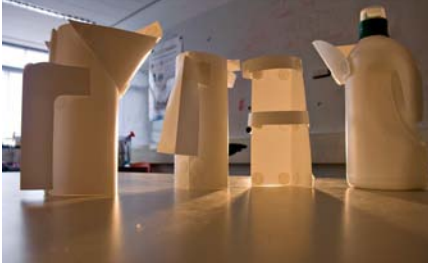
Figure 7.3. The surface modeling toolkit consists of bendable plastic sheets that can be joined using velcro stickers. The intention for the surface toolkit was that it allows fast prototyping of a shape, and offer more shape freedom than a volume modeling toolkit such as described by Sanders [Sanders & William 2001]
