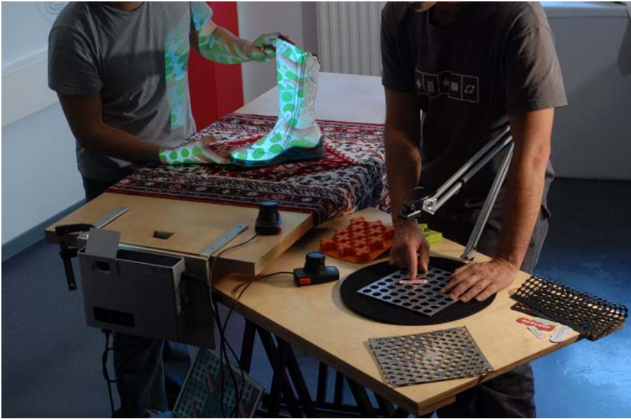
Figure 5.1. Skin in action. On the left a physical object is illuminated by a projector on the Object table. The material that is projected on the object, is mixed on the Material palette to the left. The material on the object consists of a combination of a digital background (green) and a small graphic on top of a metal sheet with holes, both captured by the camera mounted on a swiveling arm.
